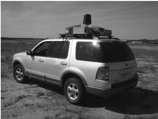
Fig. 8. Demo 2 vehicle. Mounted on the roof are three high-band antennas and amplifiers in three 120° spaced boxes. There is also a low-band switching matrix and the low-band antenna. For this second demo, the low-band was changed to a “gumdrop” antenna that contained five antennas pointing front, back, left, right, and up.
